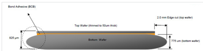
Figure 8 - Diagram of edge-trimmed, thinned wafer on carrier wafer.
