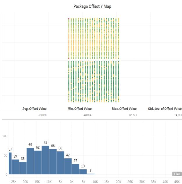
**Figure 17.** Package Position Shift in Y as measured on a panel post EMC cure
